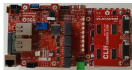
vVSP for distributed signal processing FPGA / GPU / multicore CPU / Networking / analog and digital control
