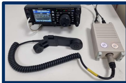
Vendor independent voice encryption for HF-radio (vHF-crypto)
